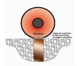
Quick Joint 85 protects concrete joint edges from wheel pressure.
